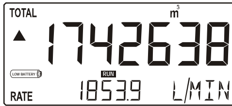
Fig. 4: Example of low-battery alarm.
